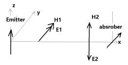
Figure 4: In this photon model, the fields  $\zeta_1 = [\vec{E}_1, \vec{H}_1, \vec{J}_1], \zeta_2 = [\vec{E}_2, \vec{H}_2, \vec{J}_2]$  do not satisfy the SCMEQ. However, they still satisfy the mutual energy principle.
