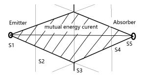
Figure 3: The mutual energy flow only exists at the overlap place of the two solutions of the SCMEQ. The field of the emitter is retarded wave. The field of the absorber is advanced wave.
