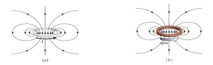
Figure 1. (a) Magnetic field around a current loop. (b) Magnetic field of a charged spinning ring
