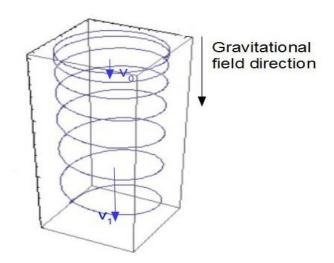
Fig.4. An OAM, |m|=1 photons descending in a constant gravitational field. The blue line represents the trajectory of a maximum intensity of the helical structure. The plot is on a length dimension axis and although the wavelength increases, because the wave-front speed also increases, the frequency increases given by the equation 2.
