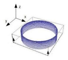
Fig.5. An internal OAM light beam m=1 slowing down to ininitesimal velocity. The black arrows represent the initial velocity of the wavefront (z=0, on z axis). At z=0, v=0 but the local beams (only the maximum intensity is depicted here) vectors still propagate at the speed of light (c).
