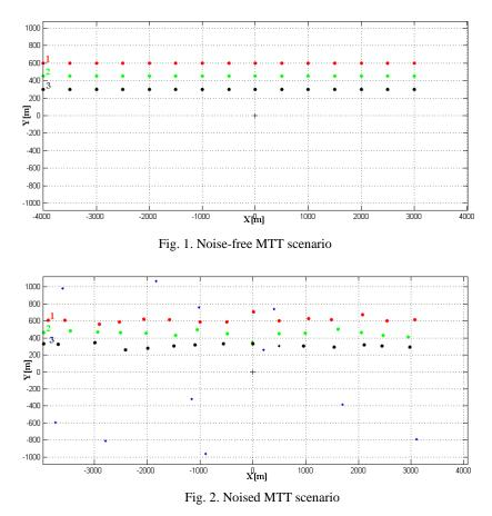
The classical target tracking algorithm was run, consisting of two basic steps: (*i*) *data association* to associate the proper measurements (distance, angle) with correct targets and (*ii*) *track filtering* to update the targets state vectors, once the optimal assignment was found. In our simulation the Converted Measurement Kalman Filter [1] is used.
