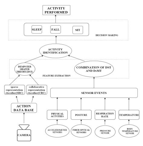
Figure: 1 Frame work for Activity Recognition
