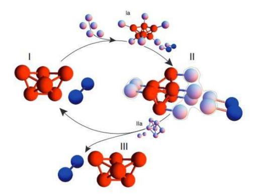
Self-Replicating Sphere Clusters: According to new research at Harvard, coating the surfaces of microspheres can cause them to spontaneously assemble into a chosen structure, such as a polytetrahedron (red), which then triggers nearby spheres into forming an identical structure.
