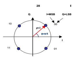
Figure 3. Bit mapping into QPSK constellation
