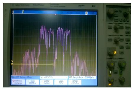
Figure 17. Signal spectrum in Rectangular Window
