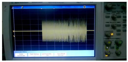
Figure 15. Received signal in time domain on DSO7032B
