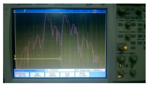
Figure 19. Signal spectrum in Flat-Top Window
