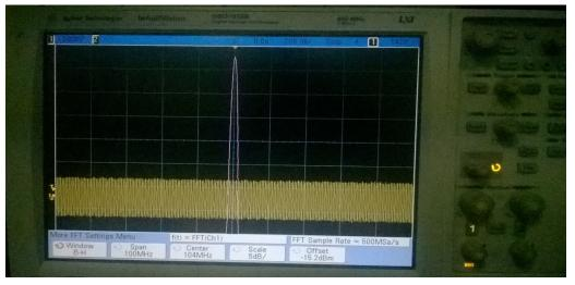
Figure 16. Peak line showing carrier frequency
