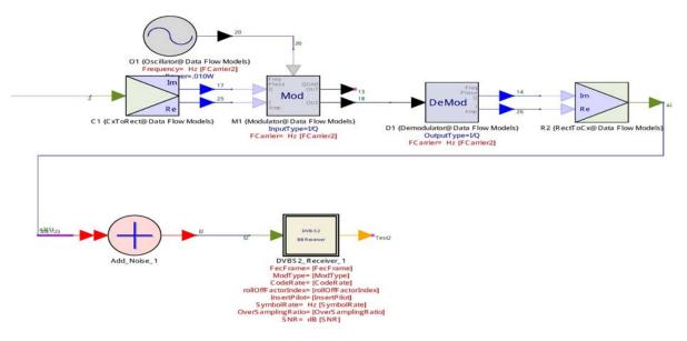
Figure 9. Implementation of Carrier Frequency Over Signal
