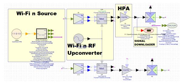
Figure 12. Wi-Fi n (IEEE 802.11N) Hotspot Design
