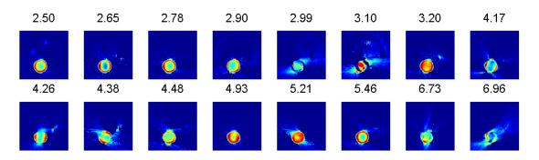
Figure 6.6: Tomographic images from ADD data of the aluminium cylinder as represented by the Gaussian area of the peaks. The numbers on the top of each image are the approximate positions of the peaks in terms of  $2\theta^{\circ}$ .
