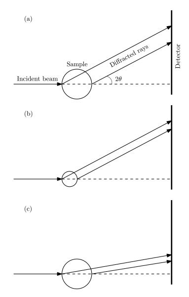
Figure 6.15: A schematic diagram illustrating the effect of sample size and scattering angle on the signal spread which is manifested in peak broadening and splitting. The large signal spread observed in (a), due to the large sample size and large scattering angle, is diminished in (b) by reducing the size of the sample and in (c) by reducing the scattering angle.
