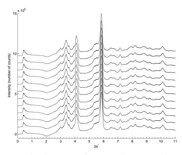
Figure 5.3: Sums of back-projected diffraction patterns for the 12 data sets of nickel nitrate reduction, presented as a stack plot.
