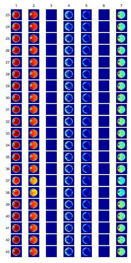
Figure 5.2: Phase distribution patterns of the nickel nitrate calcination data. The rows and columns are labelled with their indices and the background is masked.
