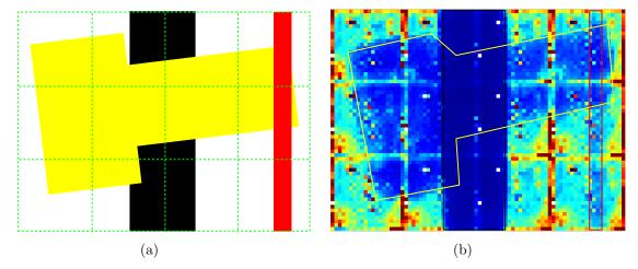
Figure 6.17: A schematic illustration (a) and a total intensity image (b) of the phantom object, obtained using the Manchester ERD HEXITEC detector. The phantom object consists of a cylinder of wax into which a bolt (yellow), a lead sheet (black) and a copper wire (red) are inserted.
