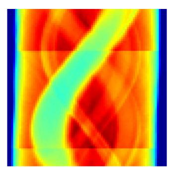
Figure 6.11: A sinogram consisting of 79 rotation rows  $\times$  80 translation columns for the EDD data. The displayed parameter is the total intensity of the individual patterns. The observed shift is due to mechanical instability of the translationrotation stage.
