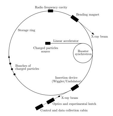
Figure 1.3: Schematic illustration of the main components of a synchrotron.
