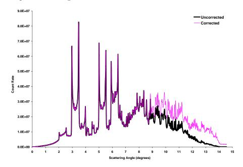
Figure 3.27: A sample of 1D diffraction pattern extracted from a 2D EDF pattern. The pink curve is obtained with the missing-rings correction while the black is obtained without this correction.
