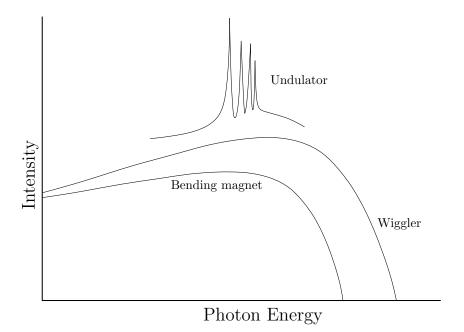
Figure 1.4: Spectra of bending magnets and insertion devices.
