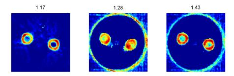
Figure 6.7: Tomographic images from ADD data of the PEEK cylinders as represented by the Gaussian area of the peaks. The numbers on the top of the images are the approximate positions of the peaks in terms of  $2\theta^{\circ}$ . In frames 2 and 3, traces of other components are masked for clarity.
