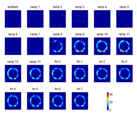
Figure 4.15: Integrated intensity of a molybdenum compound peak which is the Bragg reflection at  $2\theta = 2.10^{\circ}$  modelled by a Gaussian profile.
