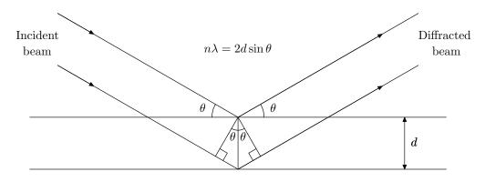
Figure 1.1: Schematic illustration of Bragg's Law.
