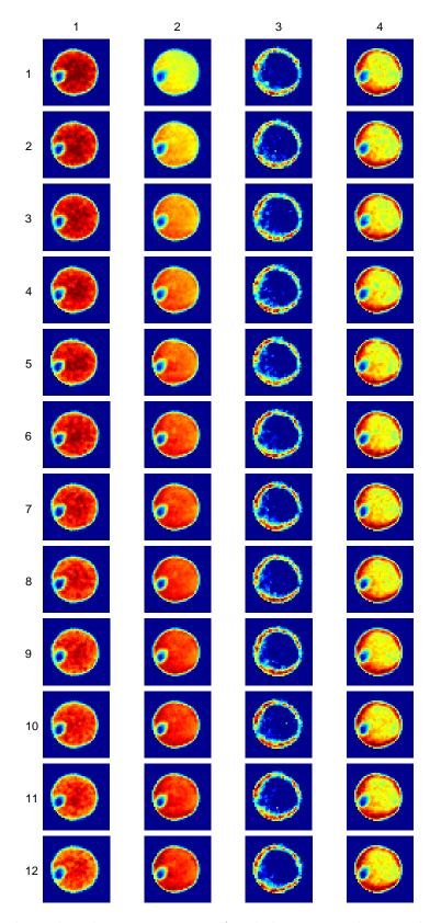
Figure 5.4: Phase distribution patterns of nickel nitrate reduction data. The rows and columns are labelled with their indices and the background is masked.
