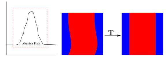
Figure 4.7: Sinogram alignment using a prominent alumina peak. The alignment matrix  $\mathbf{T}$  obtained from this operation is used to align the sinogram channels. In these schematic sinograms, blue represents the background while red represents the sample voxels.
