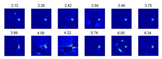
Figure 6.9: Tomographic images from ADD data of the iron oxide cylinder as represented by the Gaussian area of the peaks. The numbers on the top of the images are the approximate positions of the peaks in terms of  $2\theta^{\circ}$ .
