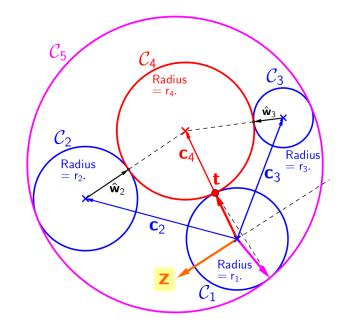
Figure 3: The geometric interpretation of Eq. (3): Our solution method has found the points of tangency of two tangent circles. One of them encloses all three of the givens, while the other encloses none of them.
