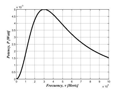
Figure.2. Power spectral distribution radiated by the *Hertz* dipole. Under these conditions, the energy of the electromagnetic radiation is given by equation (5):
