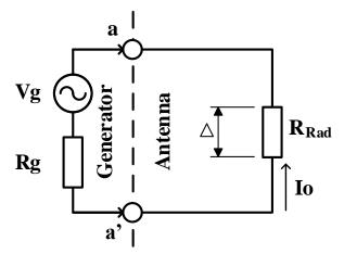
Figure. 1. Antenna-generator system.
