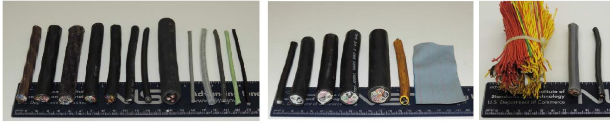
FIGURE 9. Photos of Electrical Cables Tested in HELEN-FIRE
