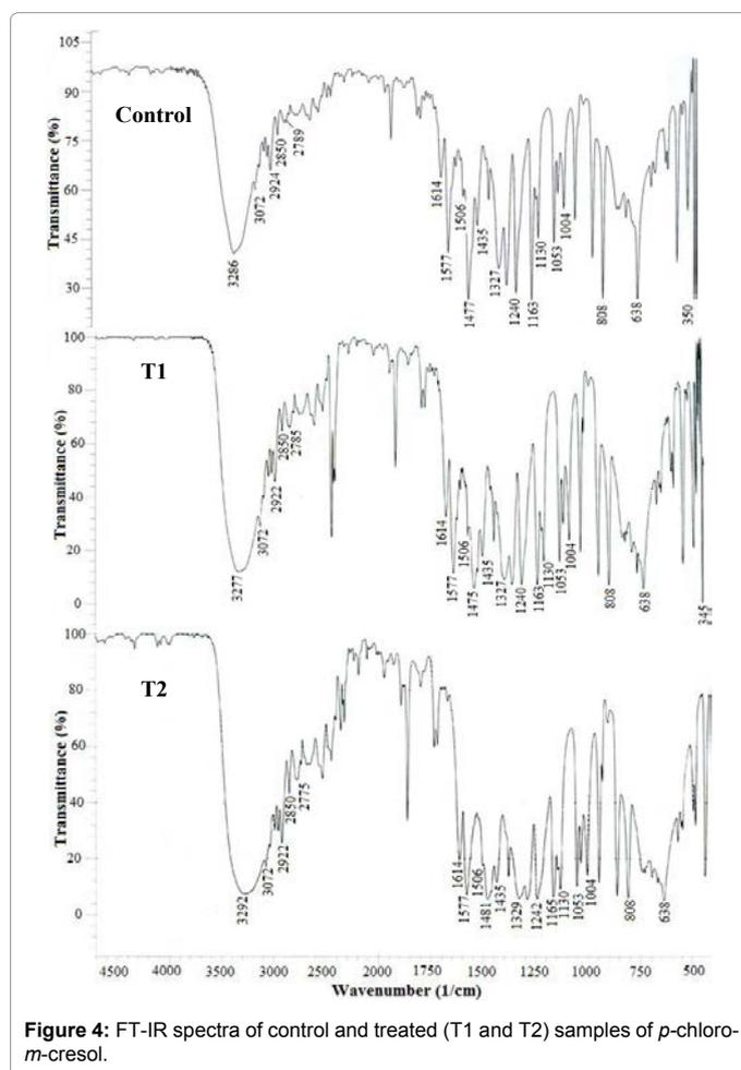
Figure 4: FT-IR spectra of control and treated (T1 and T2) samples of *p*-chloro-*m*-cresol.
