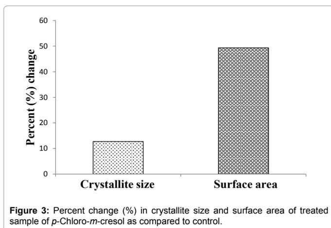
Figure 3: Percent change (%) in crystallite size and surface area of treated sample of *p*-Chloro-*m*-cresol as compared to control.
