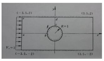
Fig. 1. Potential flow around a cylinder between two parallel plates
