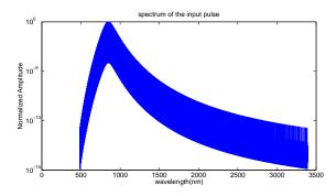
Figure 5: Spectrum of the ASK Modulated waveform with a central wavelength of 850nm
