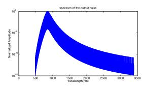
Figure 7: Spectrum of the PCF output with a central wavelength of 850nm
