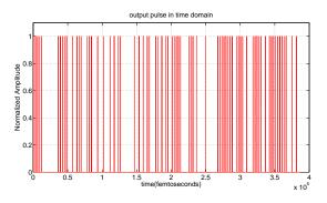
Figure 6: Output signal of the photonic crystal fiber
