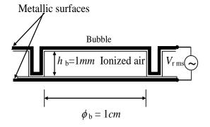
Fig.5 – Dimensions of the bubbles
