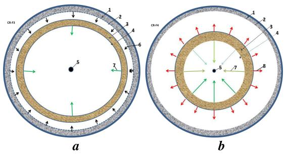
**Fig. 8**. Work of Cumulative AB thermonuclear reactor (Version 2). *Notations*: a – initial layer explosive, b – rocket part of explosive.1 -5 are same with Fig.7, 6 is pressure of initial layer of explosion, 7 is moving of explosive (force from jetted gas rocket thrust), 8 is flow of reactive explosive gas.
