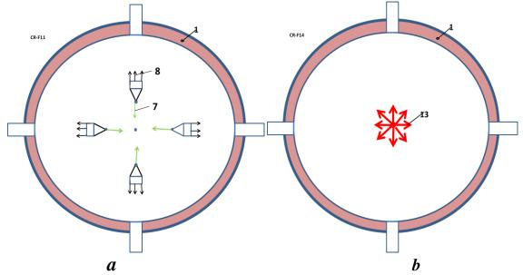
**Fig. 5**. Work of AB thermonuclear reactor (Version 1). Notations: a – rocket acceleration of pistons, b – nuclear explosion;7 is moving of explosive and pistons(force from rocket thrust), 8 is flow of rocket explosive gas. 13 – Thermonuclear explosion.
