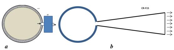
**Fig. 6.**Final (industrial) work of Cumulative AB thermonuclear reactor. Compressed gas from sphere runs to the magneto hydrodynamic (MHD) generator and produces electric energy or runs to gas turbine and produces useful work (Fig. 6a).*Notation*: 14 – conversion of hot gas pressure to electric or mechanical energy, for example, by the magneto hydrodynamic generator (MHD together with condenser), gas (steam) turbine (Fig. 6a) or moving to a rocket nozzle and produces a rocket thrust (Fig. 6b).
