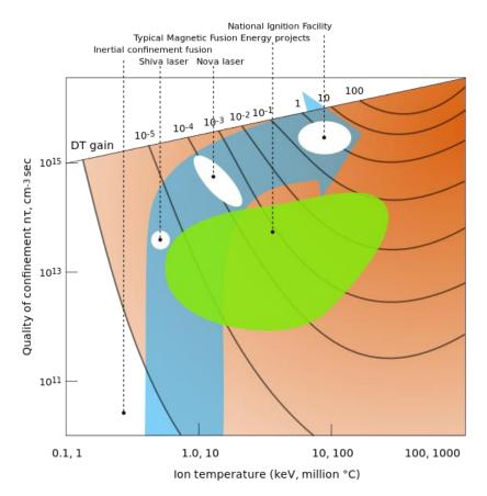
Fig. 3. Parameter space occupied by inertial fusion energy and magnetic fusion energy devices. The regime allowing thermonuclear ignition with high gain lies near the upper right corner of the plot.
