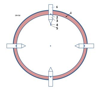
**Fig.4**. Impulse Cumulative AB-thermonuclear reactor (Version 1). *Notations:* 1 – strong sphere, 2 – fuse, 3– explosive, 4 - piston from heavy material, 5 – capsule (pellet) of nuclear fuel; 6 – tube for loading and additional initial acceleration.
