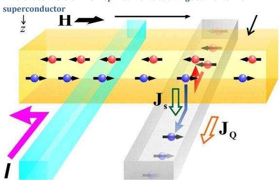
Schematic illustration of the device for measuring the SHE in a superconductor Spin injection current (I) between the ferromagnet (Py) and nonmagnet (copper: Cu) generates pure spin currents (JS) in the copper. Pure spin currents flow through the copper into a superconductor (niobium nitride: NbN), and are converted into charge currents (JQ) via the SHE inside the niobium nitride. Credit: Taro Wakamura
