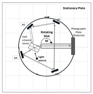
Fig.5. Schematic representation of the Sagnac interferometer
