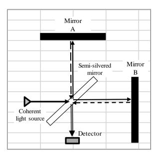
Fig.6. Scheme of the Michelson interferometer
