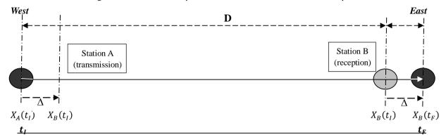
Fig.3. One-way light speed determination – eastward transmission
