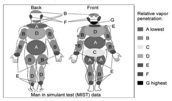
Figure 3. Vapor penetration resistance of a candidate ensemble.
