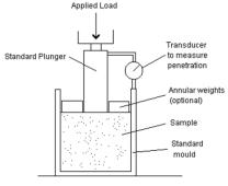
Figure. 4 Mechanism of CBR Test Machine (Gray, 1983)
