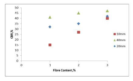
Figure. 5 results of CBR test for plastic fibre
