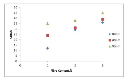
Figure. 6 results of CBR test for natural fibre
