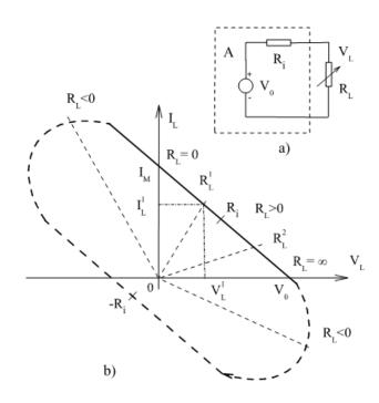
**Fig.1.** An active two-pole – a), I - V characteristic – b).
