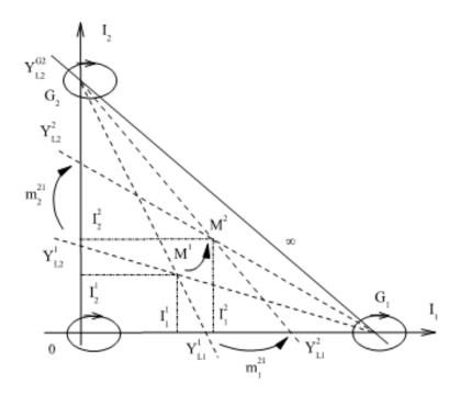
Fig. 6. Change of a regime at the expense of the load conductivities  $Y_{L1}, Y_{L2}$ .
