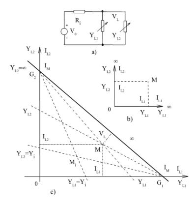
Fig.3. Simple active two-port network - a), Euclidean plane,  $R_i = 0$  - b), projective plane,  $R_i > 0$  - c).
