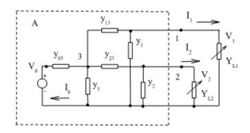
Fig.4. An active two-port network.
