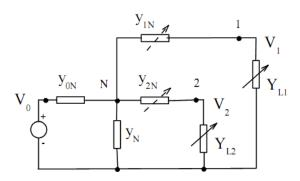
Fig. 2. Active two- port network with changeable loads  $Y_{L1}, Y_{L2}$
