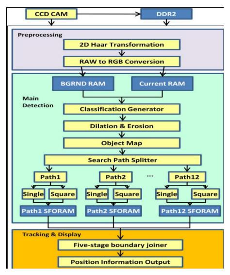
Fig.1. FPGA-Based Object Tracking System – Block Diagram.
