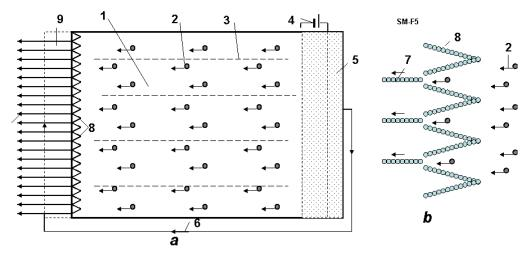
Fig. 10. Method particle traps for production of the AB-needles. *Notations*: a - device; b - particle traps; 1 - vacuum cell; 2- charged particles; 3 - magnetic lines; 4 - electric issue for the acceleration nets; 5 - plasma from particles; 6 - flow of electrons; 7 - AB-needles; 8 - trap made from AB-matter for the charged particles (p, <sup>2</sup>H, <sup>4</sup>He, etc.); 9 - cell for cover the AB-needles by electrons.
