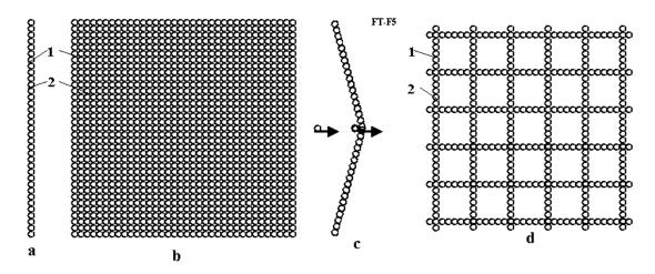
**Fig.2**. Thin film from nuclear matter. (a) cross-section of a matter film from single strings (side view); (b) continuous film from nuclear matter; (c) AB film under blow from conventional molecular matter; (d) – net from single strings. Notations: 1 - nucleons; 2 - electrons inserted into AB-Matter; 3 - conventional atom.
