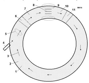
Fig. 9 Toroid producer of AB-needles (AB-matter). *Notations*: 1 - vacuum toroid; 2 - perpendicular (to sketch) magnetic lines; <math>3 - particles; 4 - particles gun; 5 - round magnetic lines from motion charged particles; 6 - electric accelerator; 7 - electric focuser; 8 - AB - needles; 9 - magnetic field keeping the AB-needles; 10 - electric focuser; 11 - electric accelerator.
