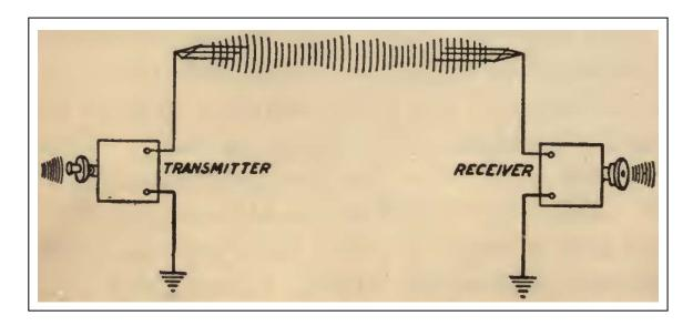
We have shown in Part II that the radio waves produced by the electric currents oscillating in the transmitting antenna are waves in the aether, magnetic in nature. The electric currents that these magnetic waves produce in the receiving antenna are due to the phenomenon of electromagnetic induction.
