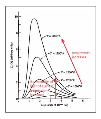
From these two observations it can be said that the effect of increasing the temperature of a hot body is to cause the atoms composing it to begin emitting light of different frequencies *in the same time*.
