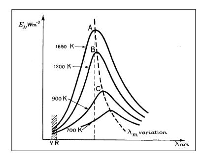
Similarly, if the temperature of the hot body is increased, the curve keeps the same shape but the total radiation (area under the graph) increases and the maximum of intensity moves towards shorter wavelengths (higher frequencies) [Robert Martin Eisberg, Fundamentals of Modern Physics, John Wiley & Sons, Inc., New York (1961), p.48]:
