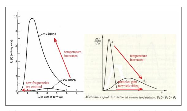
Firstly, observe that an increase in the temperature of the hot body brings about emission at new (higher) frequencies (left figure), while the distribution (right figure) tells us that at higher temperatures the atoms have greater velocities. This is consistent with the fact that at high temperatures the atoms emit more energy and do that at all frequencies because the intensity of light increases at all frequencies.
