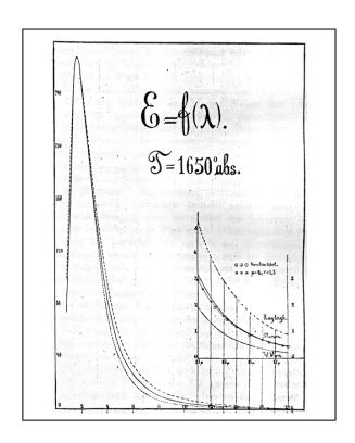
Observe that the intensity of the light emitted by the hot body does not have only one frequency (wavelength) but it is composed of a mixture of light waves of different frequencies f having different intensities.
