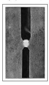
The temperature of the carbon electrodes was estimated at 3500-3900°C (for the positive) and 3000°C (for the negative). Light was emitted by the volatilized carbon burning in air.
