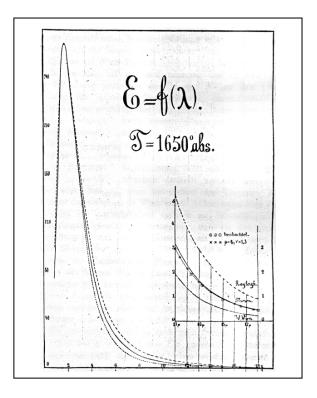
Observe that the intensity of the light emitted by the hot body does not have only one frequency (wavelength) but it is composed of a mixture of light waves of different frequencies f having different intensities.
