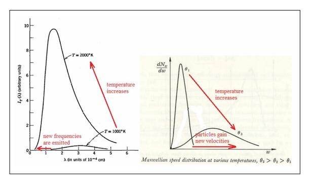
Firstly, observe that an increase in the temperature of the hot body brings about emission at new (higher) frequencies (left figure), while the distribution (right figure) tells us that at higher temperatures the atoms have greater velocities. This is consistent with the fact that at high temperatures the atoms emit more energy and do that at all frequencies because the intensity of light increases at all frequencies.
