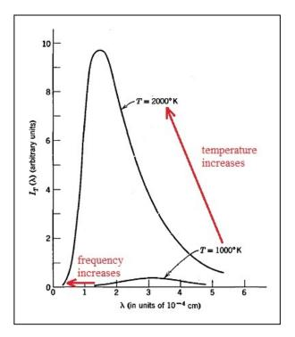
This tells us that the increase in the temperature of the hot body causes the atoms composing it to begin vibrating with higher frequency and thus emitting light waves of higher frequency.
