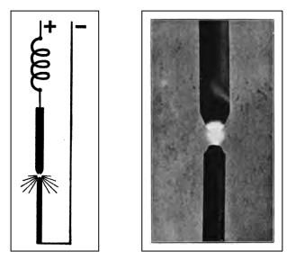
The temperature of the carbon electrodes was estimated at 3500-3900°C (for the positive) and 3000°C (for the negative). Light was emitted by the volatilized carbon burning in air.
