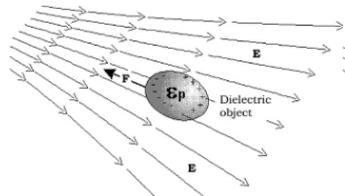
Fig. 1. Dielectrophoresis causes a particle to be attracted
