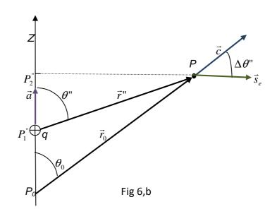
In fig 6,b we consider the case of the point charge q starting at rest in  $P_0$  and moving with constant acceleration a along the Z-axis. At the moment  $t_0 = t - \Delta t$  it is in  $P_0$  and at the moment t in  $P_1^{"}$ :  $P_0P_1^{"} = \frac{1}{2}a.(\Delta t)^2$
