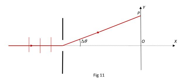
With the Huygens-Fresnel principle as starting point, we can calculate the strength of the (transversal) electric field  $\vec{E}$  in an arbitrary point in the region beyond the plate of fig 10,a.  $\vec{E}$  is an harmonic function of time.  $E^2$ , the square of the effective value of E(t), characterizes the intensity of het electromagnetic field (the intensity of light) in *P*.
