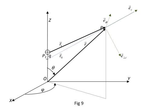
In fig 9 we consider a point charge q that harmonically oscillates around the origin of the inertial reference frame  $\boldsymbol{O}$  with frequency  $v = \frac{\omega}{2.\pi}$ . At the moment t it passes in  $P_1$ . We suppose that the speed of the charge is always much smaller than the speed of light and that it is described by:
