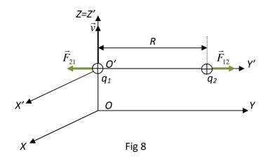
Two point charges,  $q_1$  and  $q_2$  (fig 8) are anchored in the inertial frame **O'** that is moving with constant velocity  $\vec{v} = v.\vec{e}_z$  relative to the inertial frame **O**. The distance between the charges is *R*.
