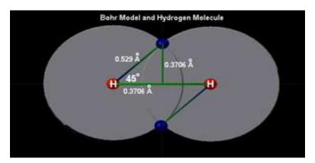
A 45-deg angle is not the optimum volley angle here, however! Unlike cannon-balls, electrons are 'electrostatically attracted to each nucleus" and "repel one another". Electrostatic energetics are minimized at the midpoint when the angle is 30-deg (see graph below).
