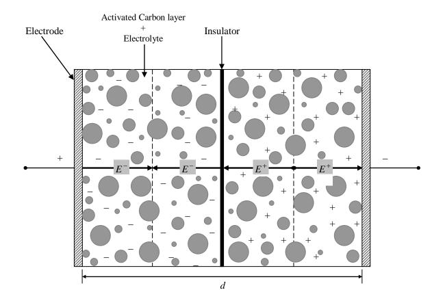
Fig. 1 – Cross-section of an *Electric Double-Layer Capacitor* (Supercapacitor) - Each *activated carbon* + *electrolyte* layer works as a *non-conducting plane of charge*, with density of charge  $\sigma^- = q^-/S$  and  $\sigma^+ = q^+/S$  respectively. The electric fields *through the layers*, due to these densities of charges  $(E^-, E^+)$ , are shown in the figure above.
