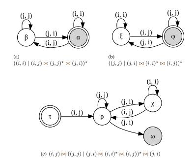
**Figure 1.** Finite state automata for the recognition of the specified regular expressions. The initial state is indicated by a double border, while the final (accepting) state is indicated by a greyed background.
