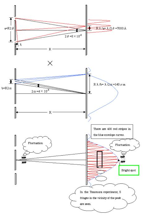
Strength of the electron wave on the screen becomes shaped like a sliced mountain. There were an estimated 400 slices in the Tonomura experiment. In addition, only a very narrow area (center part of Airy disk so-called) in the top
