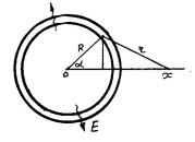
Figure 7: Two-dimensional capacitor
