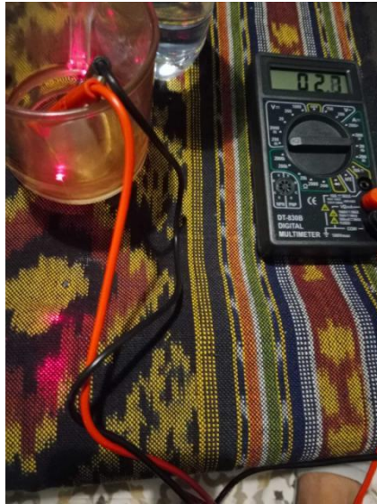
Illustration 4. Potable water irradiated with laser pen (horizontal irradiation). Note the reading at Voltmeter reads 2.7 milli Volt .
