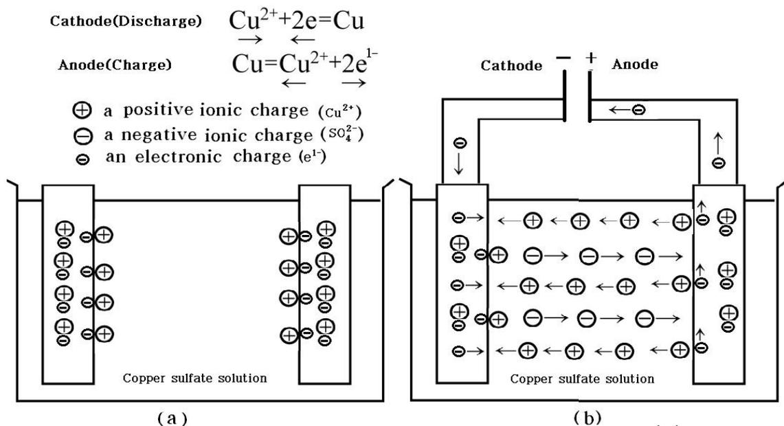
**Figure.2.** The flow mode of electric current and the material-change process at the electrodes when copper sulphate solution is an ionic conductor.
