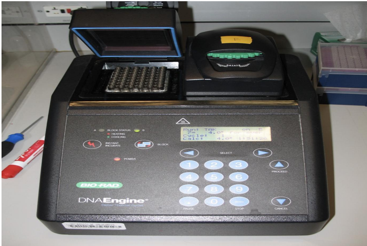
Fig. 2. A PCR machine (Bio-Rad DNA Engine Peltier Thermal Cycler)
