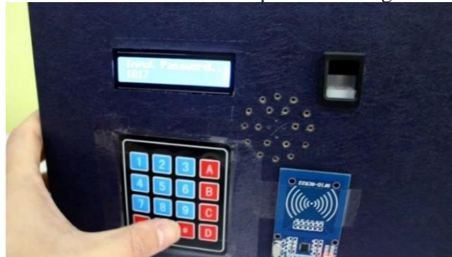
Figure 20. Password input process through 4×4 Keypad
