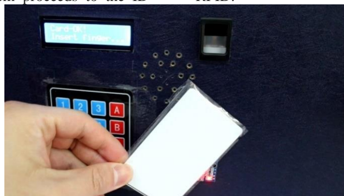
Figure 21. ID identification process through RFID
