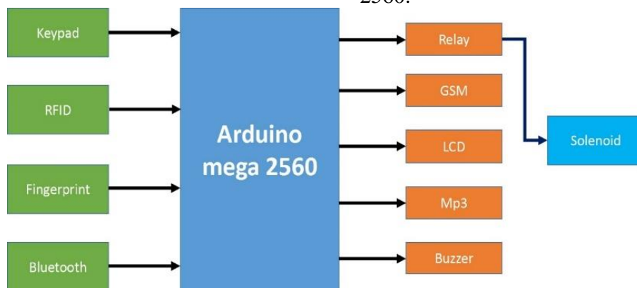
Figure 6. Configuration diagram of the quadruple security system
