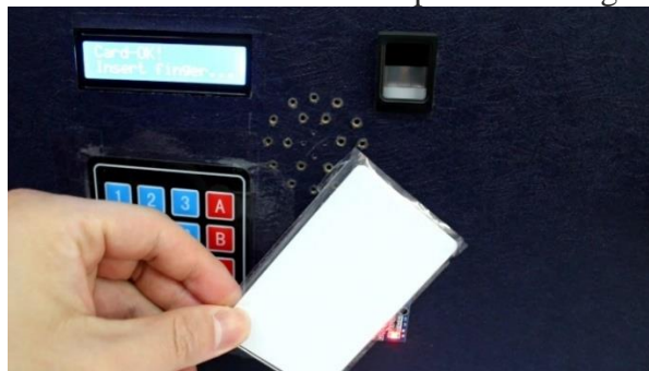
Figure 21. ID identification process through RFID
