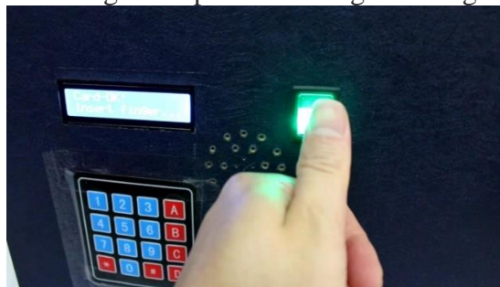
Figure 22. Fingerprint recognition process through the fingerprint module
