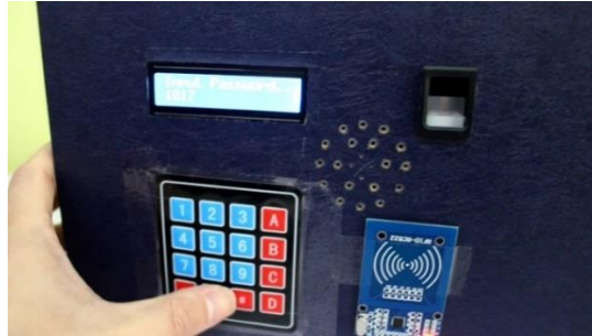
Figure 20. Password input process through 4×4 Keypad
