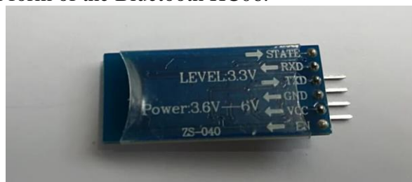
Figure 13. Physical form of Bluetooth HC 06
