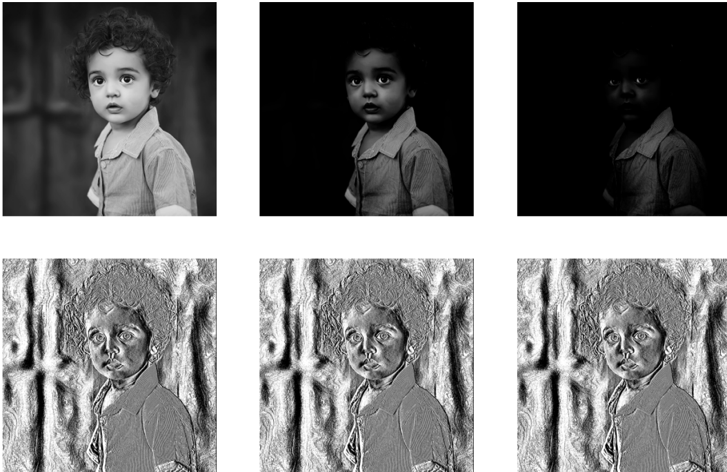
Figure 2.12: Texture images obtained by LBP under different lighting conditions [62]
