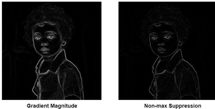
Figure 2.8: Non-maximum suppression effect on the gradient image [L]
