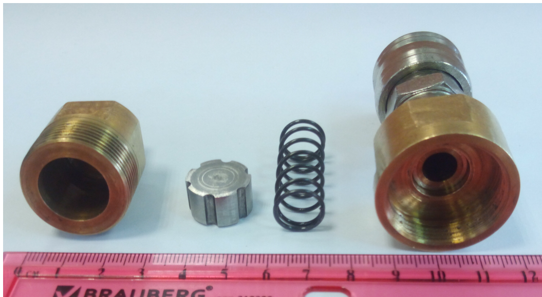
Figure 2. The exhaust valve.
