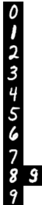
Fig.4 Incorrect case of IGC prediction. Number 9 in right side is the input image but IGC predicted number 8.
