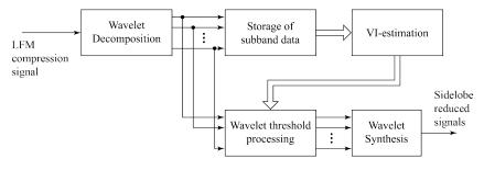
Fig. 2 VI-wavelet shrinkage adaptive processing diagram
