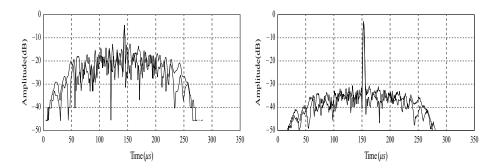
Fig. 4 PSR characteristics of LFM in the case of SNR=-10dB(a) PSR by classic method, (b) PSR by VI estimation method
