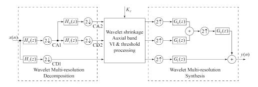
Fig. 3 Diagram of the VI-wavelet threshold processing for the sidelobe reduction
