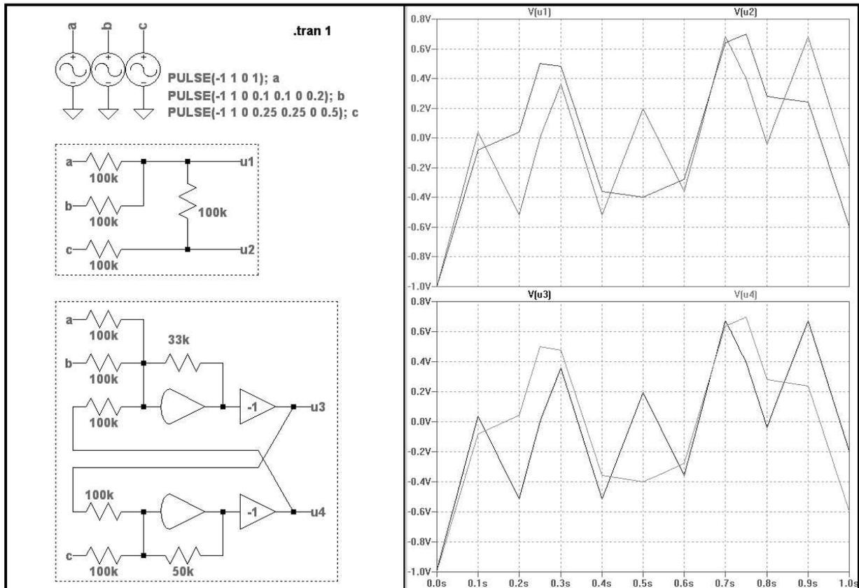
In the small box is a fragment of the DIY computer with the mutually influencing output voltages u1 and u2. Below is the equivalent circuit of an analog computer with outputs u3 and u4. Both circuits are driven with the same input voltages. Top right the plot of the two output voltages of the DIY computer. Below the output voltages of the analog computer. The results are identical.
