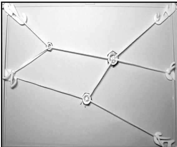
In a network of similar rubber bands and nuts, forces "superpose" and form an "entangled" overall system in which all forces compensate each other.
