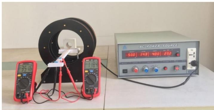
**Figure 3.4a** Electromotive force of the middle layer  $\epsilon_{LMid}$  (rms) = 0.0028 V when coil  $C_E$  is short-circuit ( $R_{LEnd} = 0 \Omega$ )
