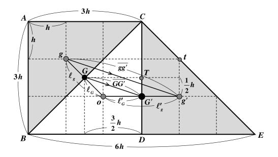
Fig. A.2.1 Movement of the centroid of whole area when a partial area moves.
