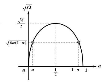
Fig. 3.2 Relationship between limiting value  $\sqrt{\Omega}$  of stable breadth and material  $\alpha$ .
