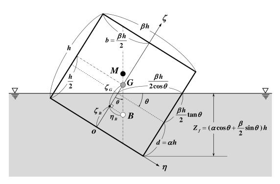
Fig. 4.1 Columnar ship, with rectangular cross-section of length *L*, floating stably in a lateral inclined state.
