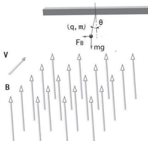
Figure 3.1 Lorentz magnetic field force of a charged moving ball in a uniform magnetic field
