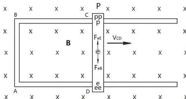
Figure 1.3 Force analysis of electrons in metal wire CD
