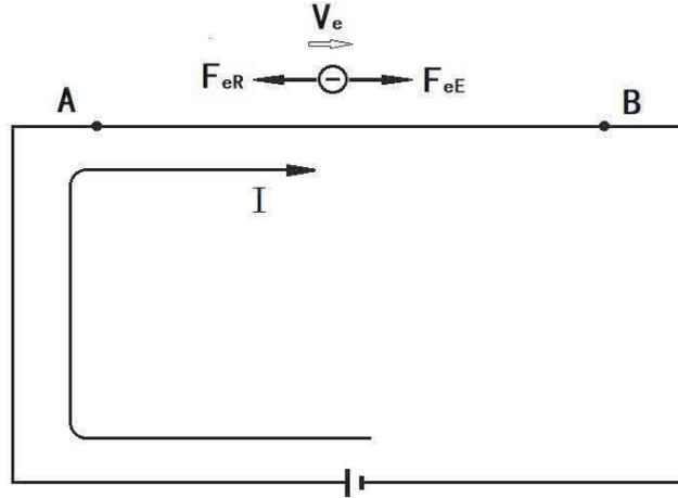
Figure 2.1 Force analysis of an electron flowing through a wire
