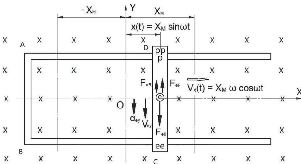
Figure 2.2 Electromotive force of wire CD moving back and forth sinusoidally
