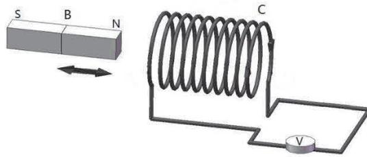
Figure 1.1 The electromagnetic induction of a metal coil
