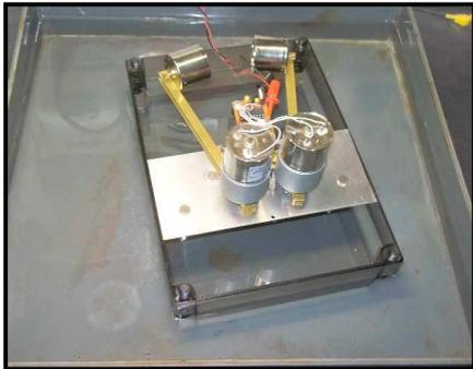
In the water bath, the weight shifts and the resulting waves forced slow movements. Because of the low friction, the return (phase 3 to phase 1) had to be slowed down. After that, the system ran perfectly.
