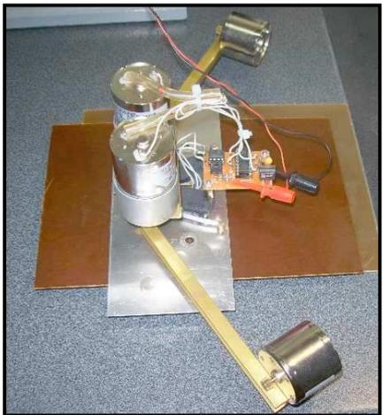
The lowest-friction and simplest method was to use free rollers between the aggregate plate and the smooth base. However, this only allows one or two cycles to be observed before the aggregate ran off the rollers.
