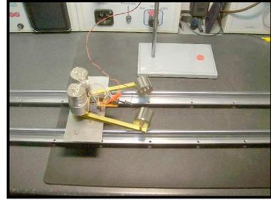
The aggregate wags its arms, to which two weights are attached, and moves jerkily to the left on the low-friction rails.
