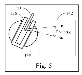
brand NaI(Tl) with an integral PMT (not shown). Gamma-rays in cone 138 must pass through scintillator 140 to get to scintillator 142.
