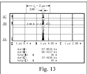
$R_e = (45/4.6 \text{ks}) - (3.6 \text{E} - 4/\text{s}) = 9.4 \text{E} - 3/\text{s}$
