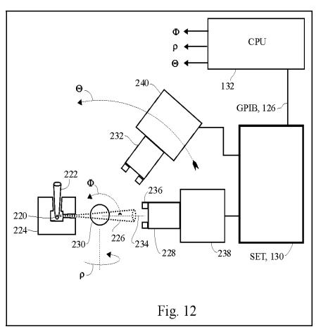
In future implementations, experimental run times can be shortened by using a stronger radioisotope source or miniaturizing the entire apparatus. Closely related is the desire to narrow cone 226 to enhance angle resolution.
