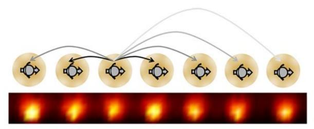
A one-dimensional chain of ytterbium ions was turned into a time crystal by physicists at the University of Maryland, based on a blueprint provided by UC Berkeley's Norman Yao. Each ion behaves like an electron spin and exhibits long-range interactions indicated as arrows. (Image courtesy of Chris Monroe)
