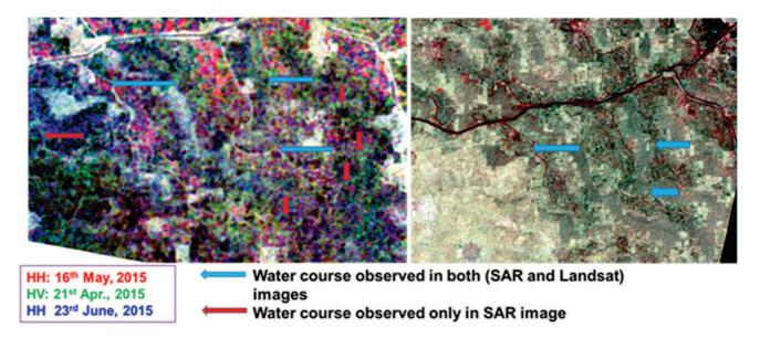
Figure 10: Multi-date Cross polarisation (HV) integrated image showing longer delineation of water courses compared to Landsat-8 image (22<sup>nd</sup> Apr., 2015)
