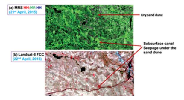
Figure 5: Dual Polarization, C-band MRS RISAT-1 image (21 April, 2015) showing canal seepage under the sand dune
