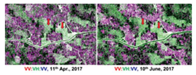
**Figure 8:** 11<sup>th</sup> June Sentinel SAR image is showing higher seepage (Green tone) as the canal is full of water as compared to the 10<sup>th</sup> Apr., 2017 image when the water supply was closed (from 27<sup>th</sup> Mar., 2017 to 16<sup>th</sup> Apr., 2017) for canal repair work.
