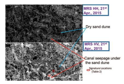
**Figure 6**: (a, upper) MRS RISAT-1 HH and (b, lower) HV polarization images (21<sup>st</sup> April, 2015). Cross polarization (HV) image showing higher sensitivity to canal seepage under the sand dunes
