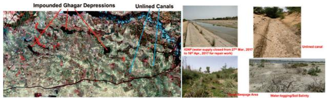
**Figure 3:** Main sources of seepage in the study area (Landsat-8, 22<sup>nd</sup> Apr., 2015)
